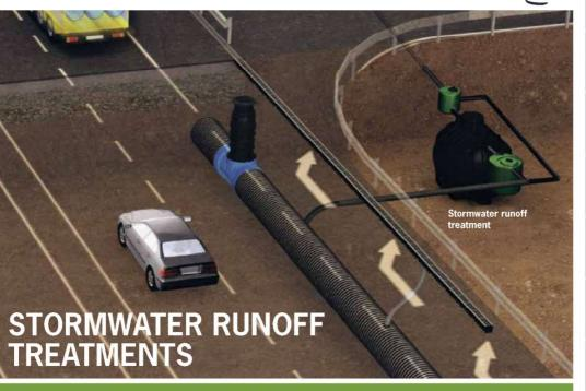
1. IPP - TREATMENT OF STORED STORMWATER RUNOFF (FROM 500 TO 12.000 M<sup>2</sup>)
